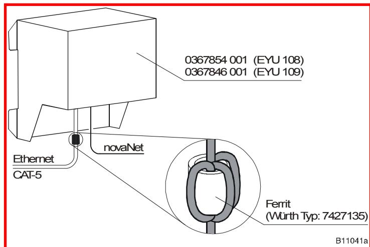
Where EN 61000-6-3 residential standard compliance is essential, three turns of Ethernet cable (min. CAT-5 cable) must be looped through a ferrite ring (Fürth type: 7427135) positioned right next to the plug. The matching front plate for the card rack must be secured. This can only be fulfilled using hardware index C.
