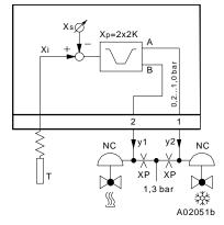
For heating and cooling: use NC valves (normally closed) (e.g. VK18P or BK18P)
